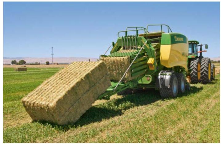
The VFS Variable Filling System from KRONE delivers rock-hard and well-shaped bales even from thin windrows and at slow forward speeds.
